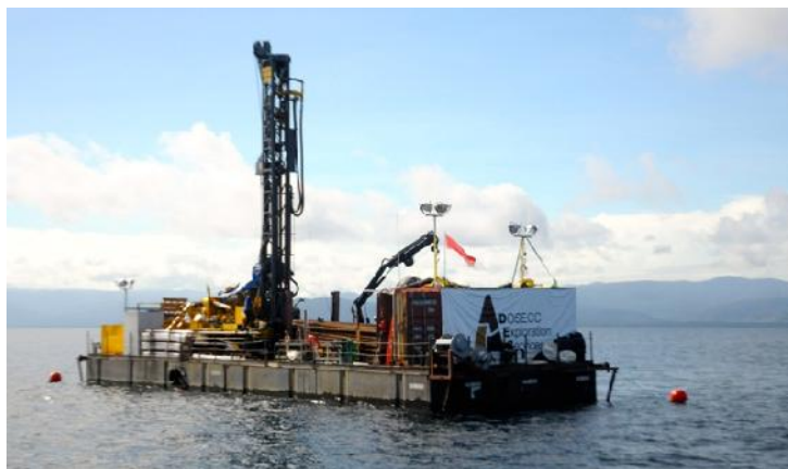
Gambar 12. Pemboran sedimen dasar Danau Towuti ( Towuti Drilling Project ) ( www.mongabay.co.id )
